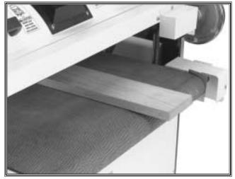
Figure 8. ALWAYS sand the workpiece with it sitting flat against the conveyor belt.
